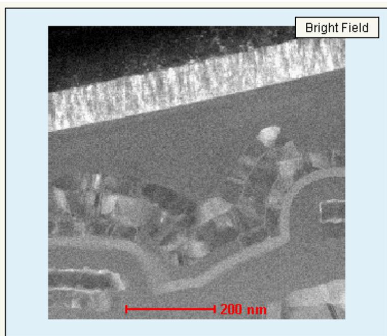
*STEM image display. At top right is displayed the detector with which the image was collected. At bottom center a scale bar is shown (in red).*
